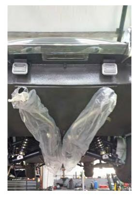
The main heat shield was fitted, allowing the exhaust (a Falcon stainless-steel system) to be fitted. Unfortunately, there was no bracket or mount for the rear tailpipes, though these were still available as spares.
