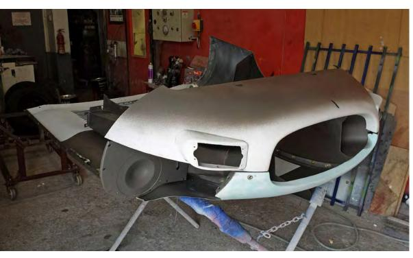
• Left: ...and now fitted to the bonnet upper section (supported inverted on trestles)...
