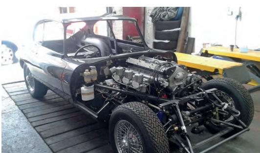
• Above left: new adjustable Gaz shock absorbers were fitted, along with the front antiroll bar
