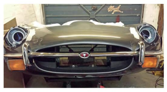
• Left: the bonnet taking shape, with front bumper, side/indicator lights and mesh radiator grille fitted
