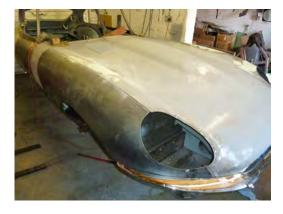
• Above: the bonnet assembly, with bumper in place, trial-fitted to the shell
