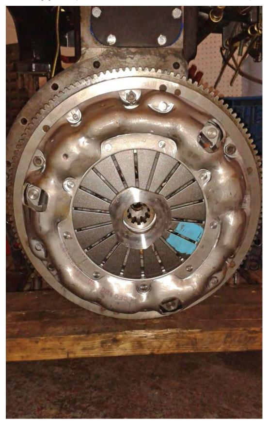
• Left: a new clutch assembly was fitted to the refaced flywheel
